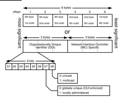
The original *IEEE 802* MAC address comes from the original *Xerox* Ethernet addressing scheme. This 48-bit address space contains potentially 2<sup>48</sup> or 281,474,976,710,656 possible MAC addresses.
